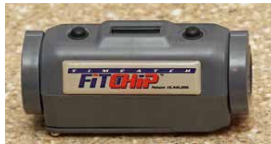
Fit Chip instrument attaches to golf club shaft to measure frequency
